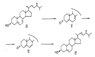
The method of obtaining brassicasterol that has been considered includes three stages and leads to the desired product with a yield of 55%, which, in comparison with the method of [12], for example, is equivalent to a shortening of the process by three stages and to an increase in yield by 30%. Thus, the proposed route to the production of brassicasterol is fairly effective and can be made the basis of the synthesis of 24R-brassinosteroids from ergosterol.
